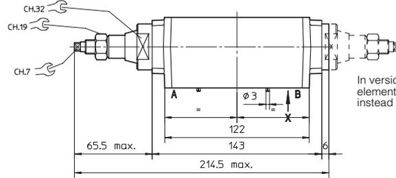
In version -214 and -224 the regulating element is on side of port B (dotted line) instead of side of port A.
