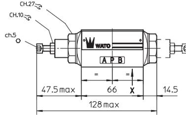
In version -014 and -024 the regulating element is on side of port B (dotted line) instead of side of port A.
