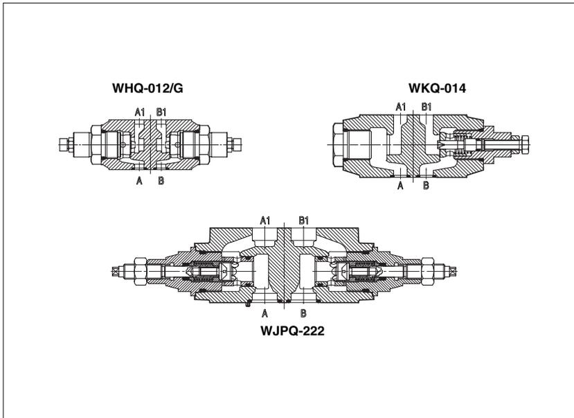
WHQ, WKQ and WJPQ are flow throttling valves, not compensated, and with check valve to allow free flow in the opposite direction.
