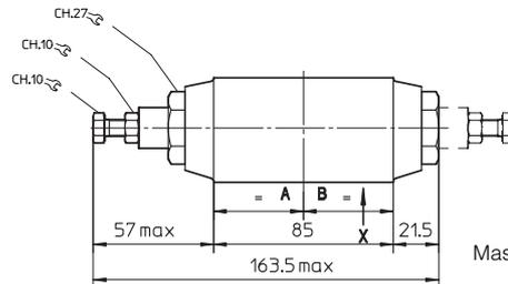
In version -014 and -024 the regulating element is on side of port B (dotted line) instead of side of port A.
