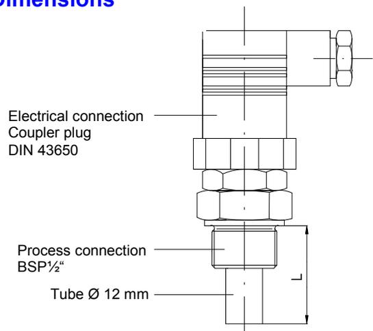
L = Total length from sealing face of process connection
